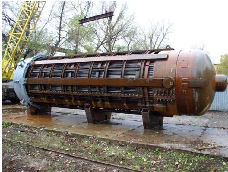
Fig. 3 Tube Bundle of Vertical Waste Heat Boiler
