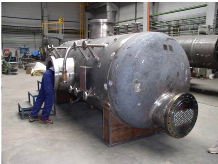
Fig. 7 Waste Heat Boiler at Fabrication
